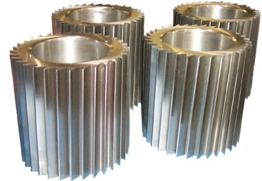
Rotor Repair and Re-sharpening
