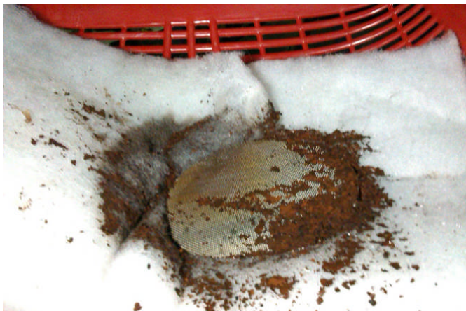
Scales and Rust pickups (inside cooling channel of barrels) at the end of service (not including dissolved scales in chemicals – dissolved scales in chemicals is estimated to be around 0.5kg)
